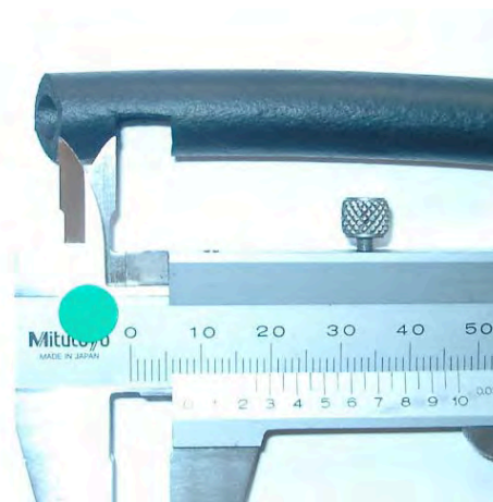
Drainage channel web width = 7 mm
