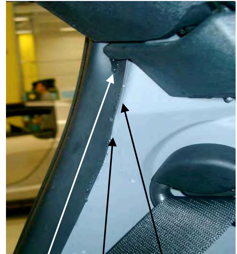
Water via inner liner
