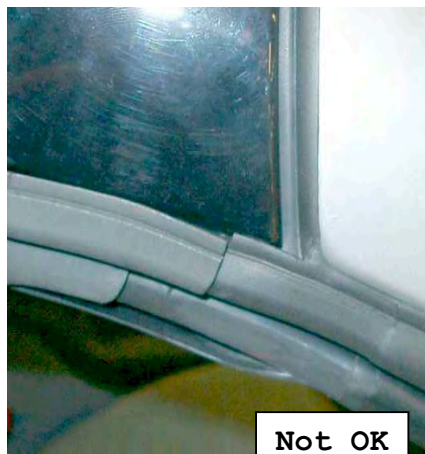
Seals in contact with one another and compressing
