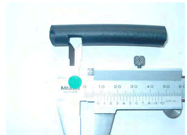
Channel notch = 8 mm
