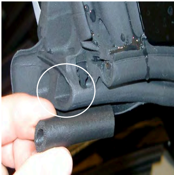
Insert hose (l=40mm)...
