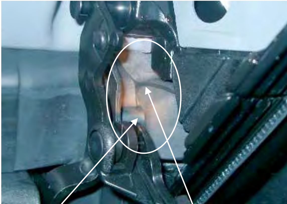
Canopy seal blow pipe, wasser exiting from canopy trough
