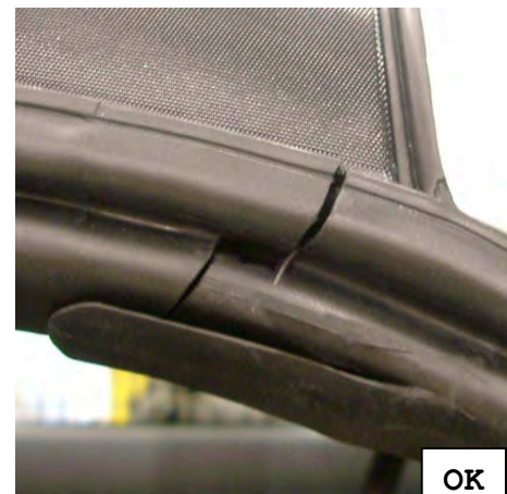
The seals sit flush side by side, Width of joint approx. 1 - 1.5mm
