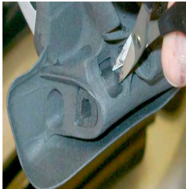
...mark the exact position of the drainage hole...
